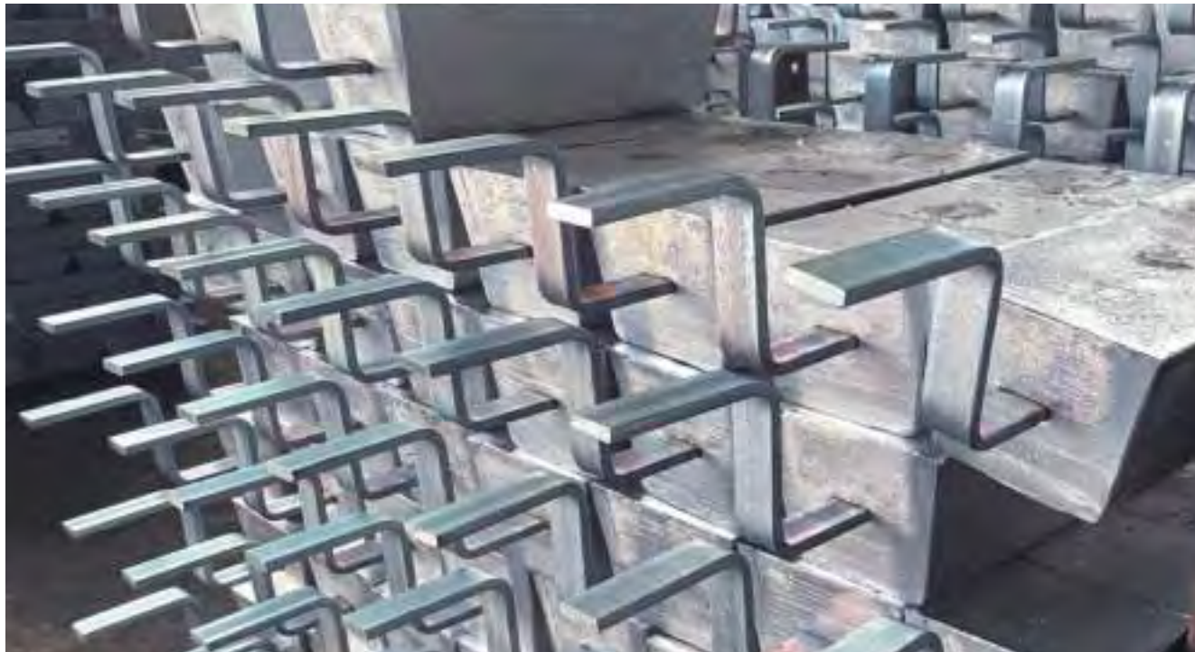
Anode with Cranked Flat Bar Insert Protruding from Both Ends
