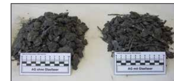
Asphalt granulate without glass fibres (left) and with glass fibers (right)
